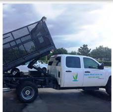
**Dump trucks** are built to haul heavy loads and dump them easily. When debris is removed from a site, a dump truck is ideal for hauling and disposing of debris.
